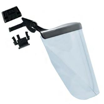
Provides protection against particles of moderate energy and moving at 120m/s, and liquid and molten metal splashes, and also arcing. Optical properties of the shield meet requirements of optical class 1 (the highest).
