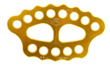
Rigging plate enables perfect alignment of connectors in the line of action of the force. It can also be used as a main rigging point in complex systems. The rigging plate has 5 holes 20mm dia at one side, and 8 holes 20mm dia for connectors.
