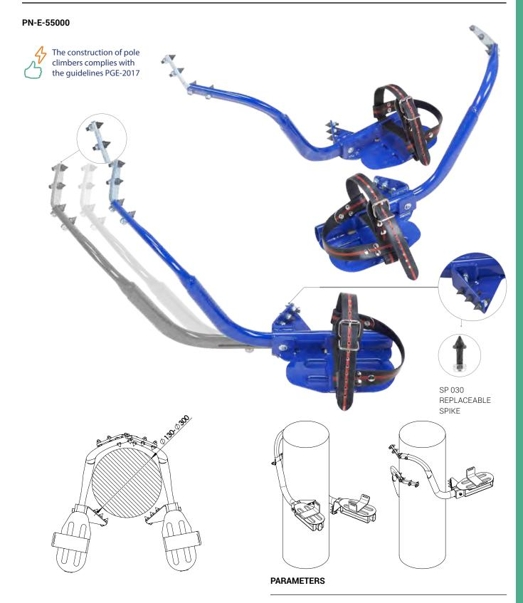
Pole climbers for wooden poles type D with variable adjustment are suitable for use on wooden poles sized 130–300mm. The device is fitted with replaceable hardened steel spikes.
