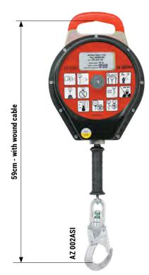
Retractable type fall arrester CR 210 in steel cover with expandable galvanized steel 4 mm cable. The device is intended for works requiring significant mobility in respect to attachment point. Energy absorber is not required...
