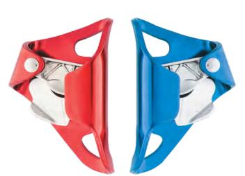
Chest ascender CD 201 ultra light and CD 202 ultra light without handle is designed for rope ascending or belaying. To be used with a kernmantle rope 8-13mm dia. Fitted with rope grab.
