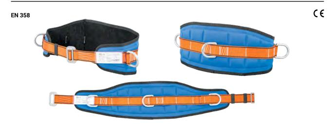
Belt fitted with ergonomically profiled padding, connecting and adjusting buckle, side attachment buckles and dorsal attachment buckle. Work positioning belt PB 11 complements fall protection equipment and prevents falls from height during works at poles, trees, building structures, etc.
