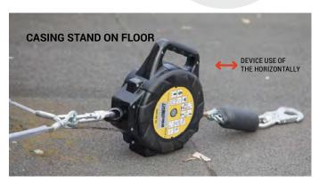
Self-locking device CR 250HV + G for vertical and horizontal operation with a pull-out safety rope and a swivel mounted in a casing made of a conductive plastic with an earthing conductor. The device has an additional shock--absorbing system located near the snap-hook. No need to use a safety shock absorber and no need to use an AZ 800 cord attached during horizontal wor.
