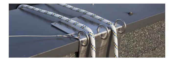
AX 902 are guards providing protection of roof parapet elements and rope or webbing against sharp-edged parapet elements. Parts are made of stainless steel. The parts are suitable for use with one textile rope or webbing. The device is mounted to structural elements by connectors AZ 011.
