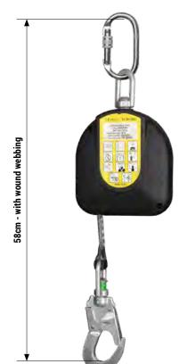
Retractable type fall arrester WR 100 with connectors AZ 011 and AZ 002ASI, fitted with expandable webbing, 17mm wide. Locking mechanism inside the composite cover. The device is intended for works requiring mobility in respect to attachment point. Energy absorber is not required.
