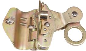
Guided type fall arrester AC 012 intended for use with work rope AC 100, 14mm dia. Parameters of the device enable direct connection to full body harness – with no energy dissipater required.
