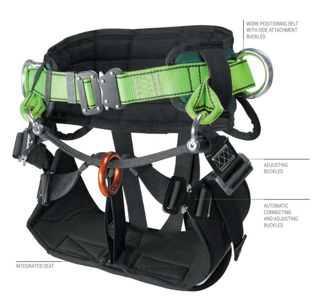
Work positioning belt for tree climbers TH 50 with an integrated seat. Equipped with ergonomically profiled padding, adjusting buckles, side attachment buckles and attachment point for work in a harness complying with EN 813. The belt includes automatic connecting and adjusting buckles Comfortable wearing and removal. Belt TH 50 is a basic equipment for works at height, mainly at trees, poles, building structures, etc.
