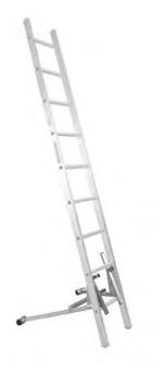
Ladder stand DS 801 is designed for supporting a single ladder max. 2.5m long. To keep stability, the ladder working height should not be greater than 1.6m.
