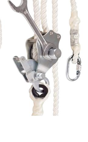
Adjustable horizontal lifeline (horizontal fall protection line). Fitted with loops with thimble at both endings. Line length adjuster (tensioner) is made of galvanized steel. To be used for works requiring frequent mobility in the horizontal. Horizontal lifeline AE 300 complies with EN 795 (portable anchor points for fall protection equipment). In order to connect horizontal anchor line AE 300 to full body harness, use an energy absorber with lanyard only. Line tensioning wrench included.
