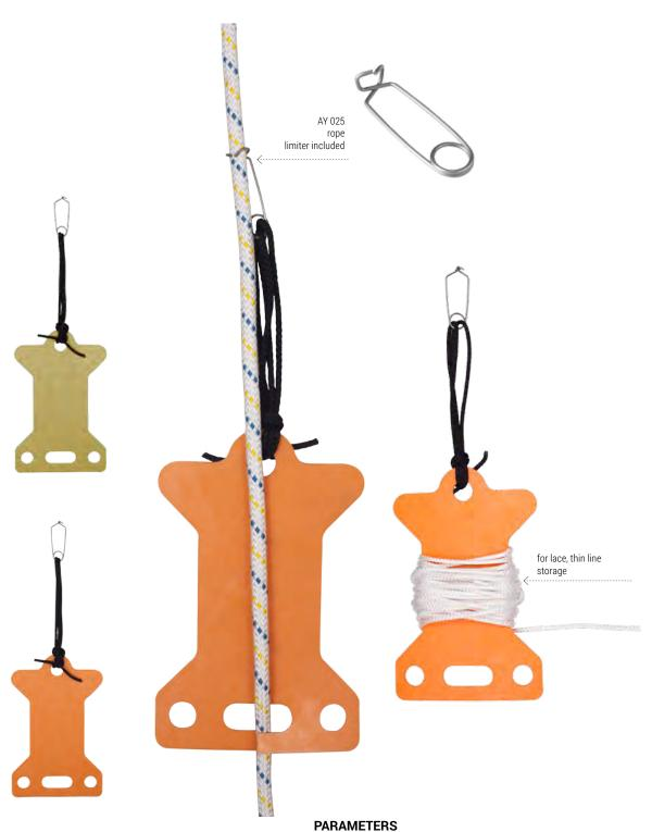
The TU 323 pad is designed as a multifunctional patch enabling i.e. comfort storage of laces and thin lines, protecting sharp edges when using lifelines, guarding rope ends against damage by pulley blocks, etc.
