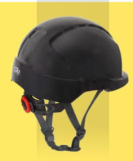
ATRA10 is a helmet that meets the highest electrical insulation standards. It protects against accidental, short-term contact with a live conductor up to 440V AC (in accordance with the optional requirements of EN 397) and can be used as an electrically insulating helmet
