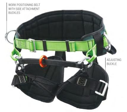
Work positioning belt for tree climbers TH 20 fitted with ergonomically profiled padding, adjusting buckles, side attachment buckles and attachment point for work in a harness complying with EN 813. The belt includes aluminium adjusting buckles. There is no risk of an accidental release. Belt TH 20 is a basic equipment for works at height, mainly at trees, poles, building structures, etc.
