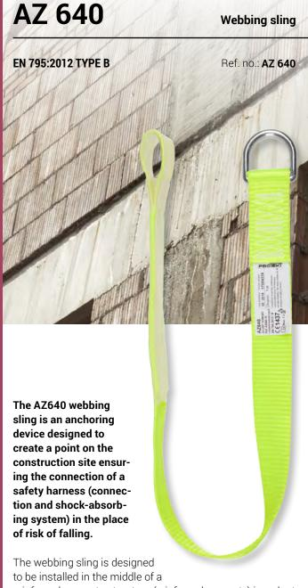
reinforced concrete structure (reinforced concrete) in order to create a point for fastening safety harnesses and permanent horizontal safety systems. The webbing sling is intended for use by only one employee. The device has been tested and positively certified in accordance with EN 795: 2012 (Fall protection from height, Anchor devices, Requirements and tests, TYPE B). The webbing sling can be used with a self-locking device, in accordance with the EN 360 standard.
