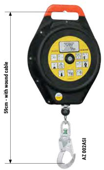
Retractable type fall arrester CR 300 with expandable galvanized steel 4mm cable. The device is intended for works requiring significant mobility in respect to attachment point. Energy absorber is not required. The device is tested and approved for working on flat roofs in combination with roof lanyard AZ 800.
