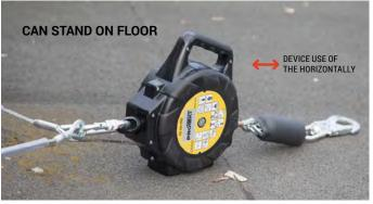
CR 250H + V self-locking device for vertical and horizontal operation in a plastic casing with a pull-down steel rope and a swivel mounted in the casing. The device has an additional shock-absorbing system located near the snap-hook. It is intended for work requiring considerable displacement in relation to the point of attachment. No need to use a safety shock absorber. No need to use AZ 800 cable when working horizontally.
