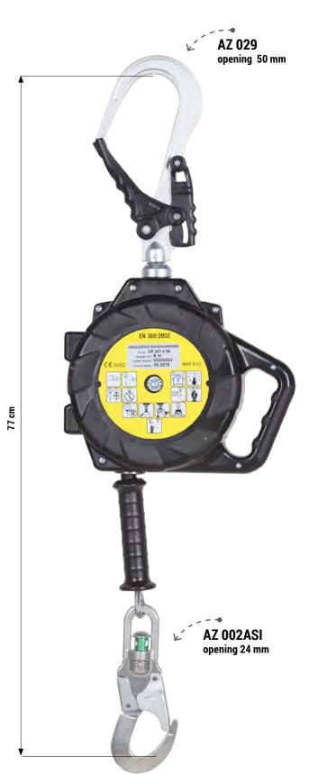
CR 251V retractable fall arrester provided with plastic housing and wire rope. Provided with AZ 029 hook with an opening larger than the standard snap hook - 50 mm (used to attach directly to the fixed structure). Device is designed for work requiring significant displacement in relation to the point of attachment. No need to use a shock absorber.
