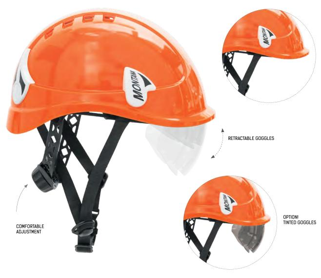
Protective helmet is made of polycarbonate which provides its resistance to damage and very low weight. The helmet is comfortable in use, and fits to the head shape and size – it is fitted with six-point webbing harness and includes a sweat band. Has closable ventilation holes. At both sides, slots for mounting hearing protection are provided..
