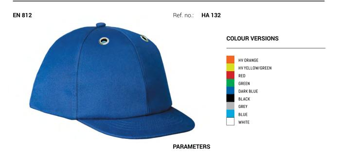
Light industrial safety helmet with protective pad. Provides head protection against impacts by solid objects or structural elements. Not suitable for protection against falling objects. Size adjusted by adjustment strap at the back.
