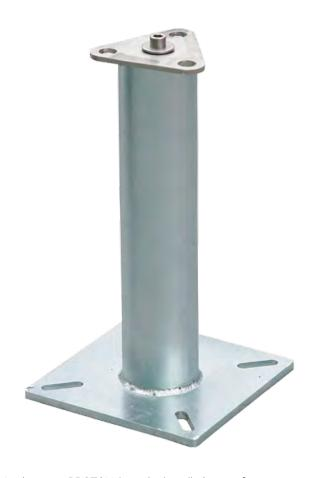
Anchor post PROTON 1 can be installed on roofs, terraces, platforms and beams. It is fitted with a three-hole plate enabling connection of personal fall protection equipment. The device complies with EN 795 type A.
